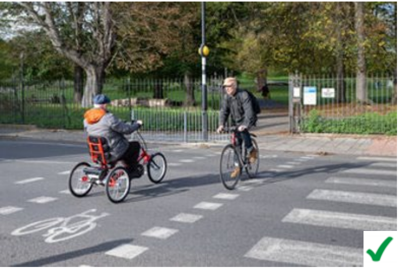
Alignment of railings permits comfortable park access to legitimate users
