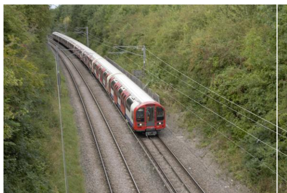
Figure 4: AC Traction dynamic testing at an off-site test track
