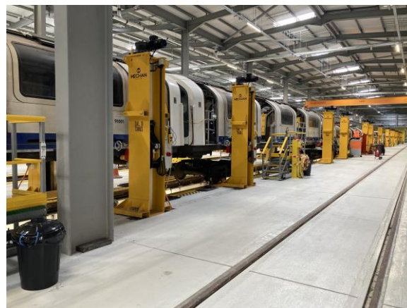
Figure 7: First CLIP pre-production train being lifted at TMU, Acton
