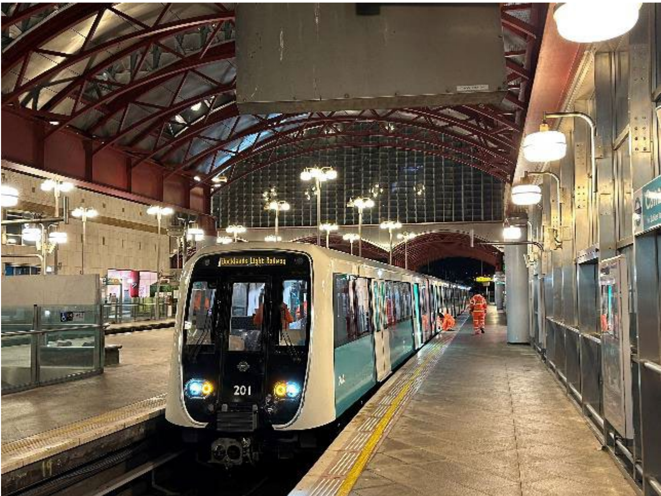
Figure 49. First new DLR trains under test at Canary Wharf station. Source: TfL.
