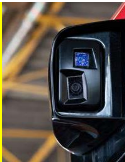
Camera monitoring system camera
